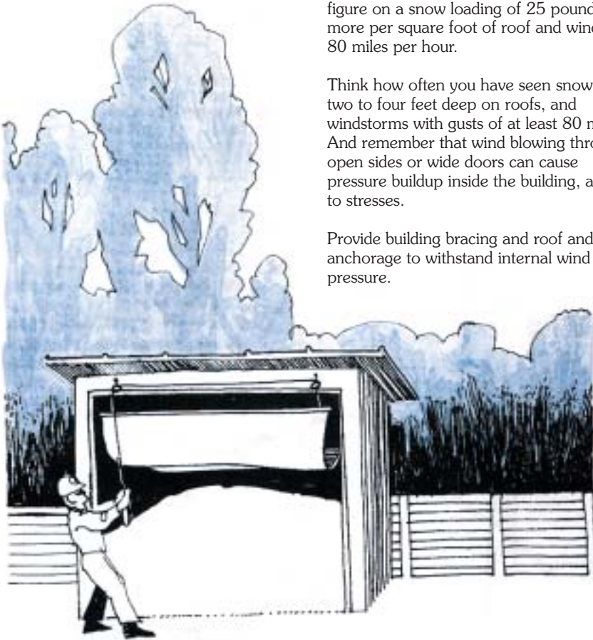
Provide pull-down cover for open-end storage buildings; one method is shown here.
