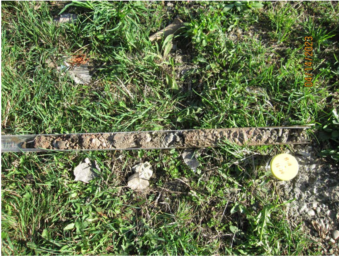
Photo 25: FILL materials observed from B-10a (16-20).
