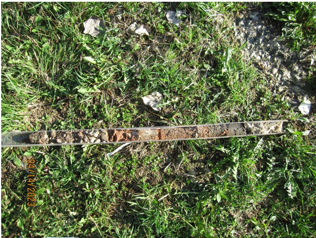
Photo 24: FILL materials observed from B-10a (12-16).
