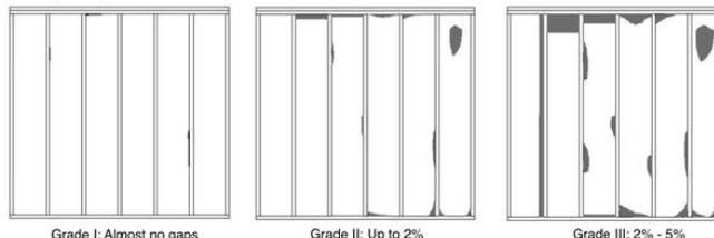
RESNET protocol for the effect of missing insulation on installation grade
