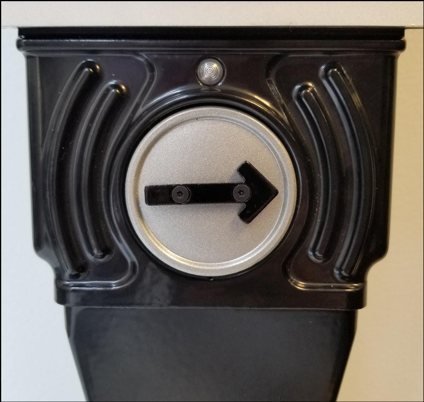
Figure 2 - APS pushbutton with vibro-tactile arrow and pilot light
