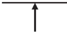
Mark will be from line to centerline of package or pipe with denotation of above symbol.
