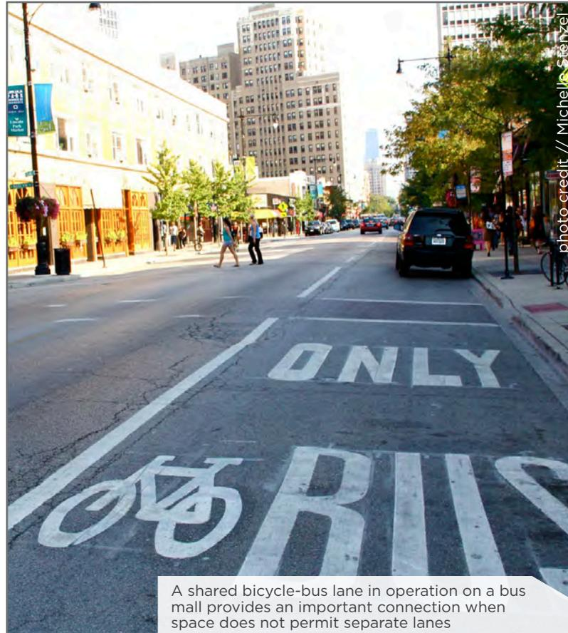
A shared bicycle-bus lane in operation on a bus mall provides an important connection when space does not permit separate lanes
