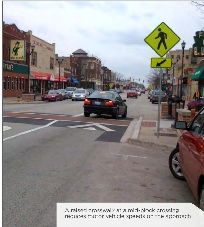
A raised crosswalk at a mid-block crossing reduces motor vehicle speeds on the approach
