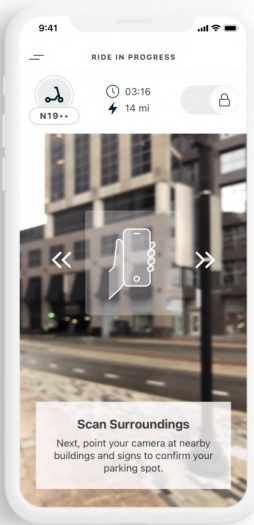
4. Scan Surroundings: When the phone is pointed up, we direct riders to scan buildings to the left and right. We use these images to triangulate their precise location.
