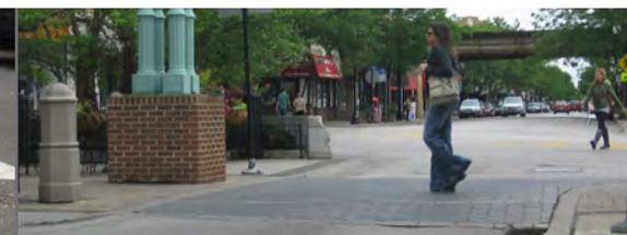
A speed table and a raised intersection are essentially longer speed humps used to raise the crosswalk or intersection and reduce vehicle speeds.
