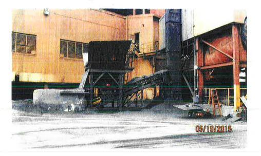
COMMENTS: Photo#4 Direction: NW Comments: Particulate dust accumulations around the silo feeding and bucket elevator.
