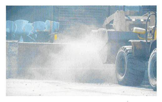
COMMENTS: Photo#1 Direction: SE Comments: Dust and particulate emissions from Ferrous Silicon(FESI)unloading operations from rail cars.
