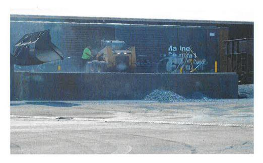
COMMENTS: Photo#3 Direction: SE Comments: Dust and particulate emissions from Ferrous Silicon(FESI)unloading operations from rail cars.
