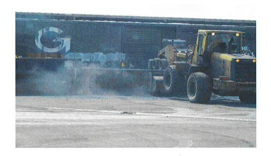
COMMENTS: Photo#2 Direction: SE Comments: Dust and particulate emissions from Ferrous Silicon(FESI)unloading operations from rail cars.
