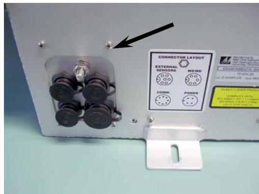
4. Remove the entire E-Sampler internal assembly from the enclosure. You will have to unplug the temperature sensor harness from the PCB, and unplug the exhaust tubing from the exhaust port in the bottom of the enclosure. Note the connector locations.
