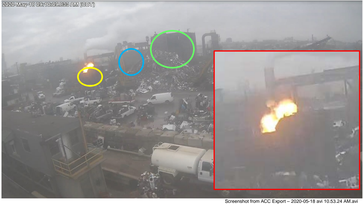
Figure 3. Screenshot from provided video at 9:10:09:833 AM. The approximate location of the RTO is circled in yellow, the filter in blue, and the shredder in green. A first appearance of flame above the RTO is visible in the enlarged inset outlined in red.
