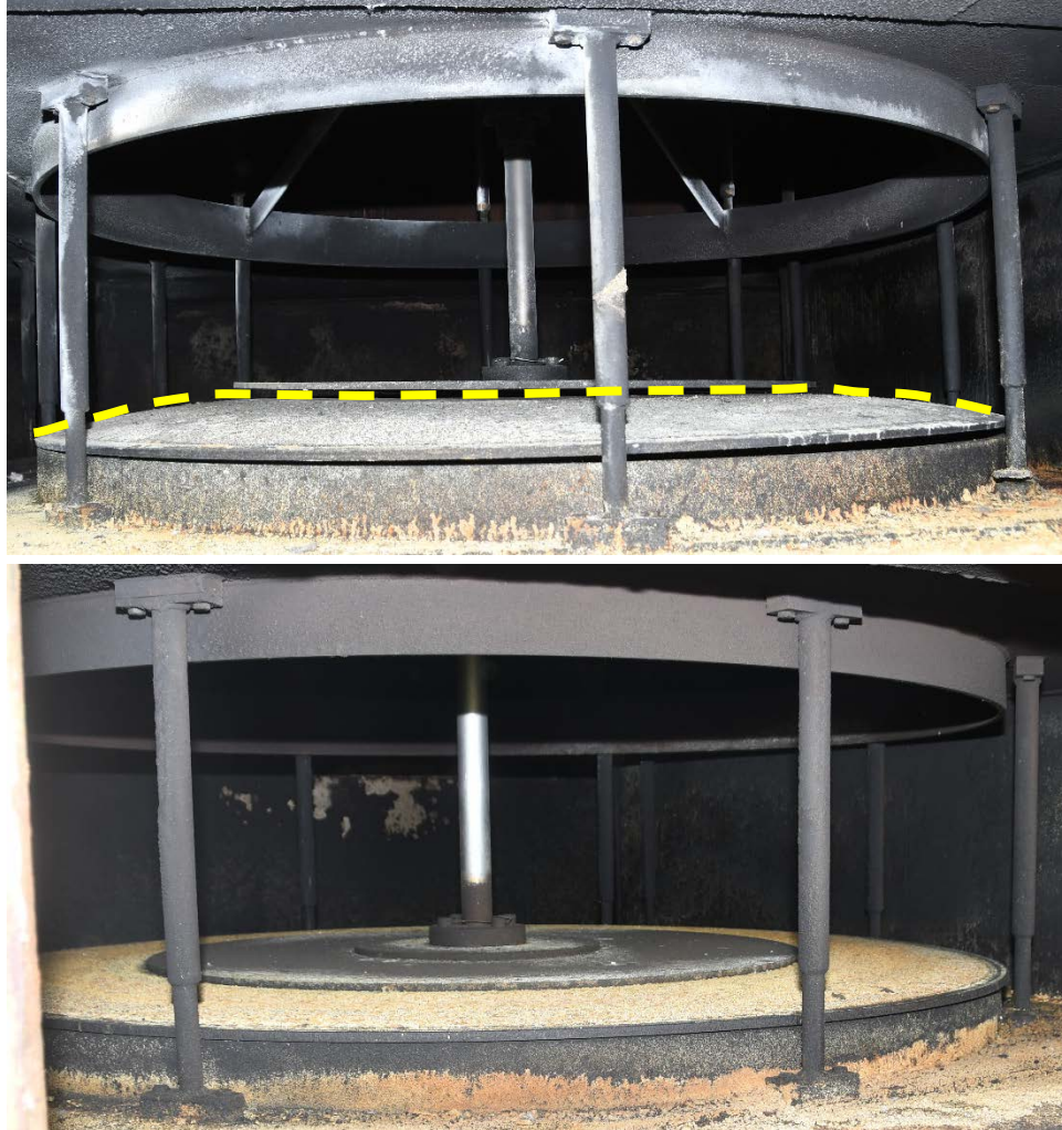
Figure 8. Photographs of one of the south poppet valves (top) and one of the north poppet valves (bottom). The south poppet valve appears to be deformed as indicated by the dotted yellow line whereas the north poppet valve is flat.
