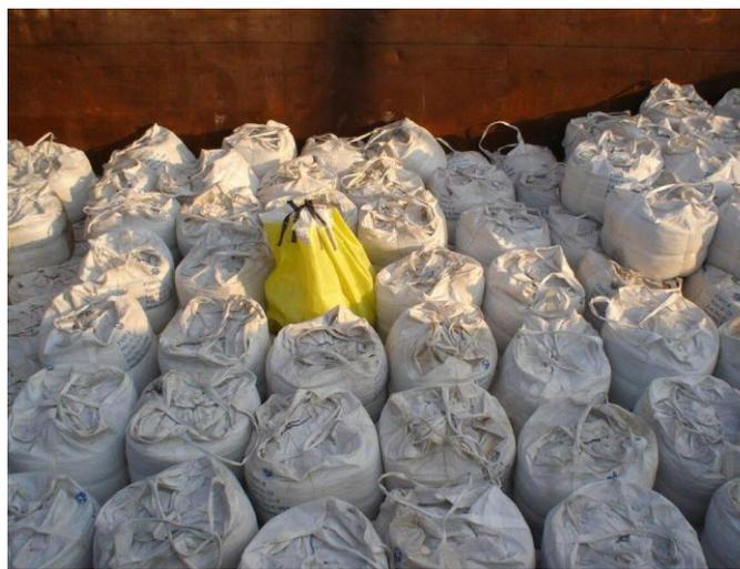
**Image 1:** Unloading of “Super Sacks” from barge. Due to the density of the products handled, such as the Magnesite contained within these “Super Sacks” the barges we handle appear to be barely full and are not traveling with product above the side walls of the barge.
