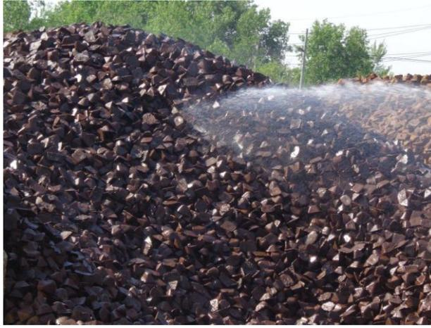
**Image 14:** Watering Pig Iron pile. Note the difference in color between the pile that is being sprayed and the dry pile in the background.
