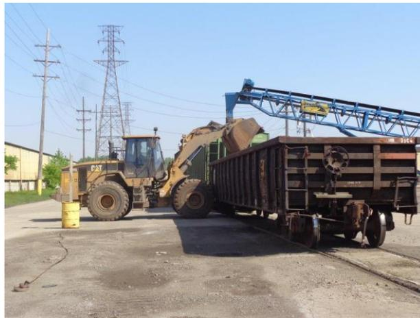
**Image 9:** Loading an open gondola rail car with Pig Iron. Note the front end loader is operating on a concrete pad and no fugitive dust is present. The Pig Iron was sprayed with water prior to handling.
