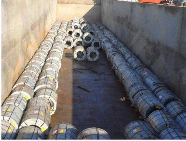
**Image 2:** Steel Coils awaiting unloading from a barge. Material arrives banded and covered to prevent damage, no fugitive dust associated with this product category. Note the cleanliness of the barge.
