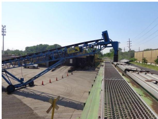
**Image 10:** Loading proppants sand into a covered hopper rail car. Note the conveyor chute is lowered inside of the rail car, limiting exposure.
