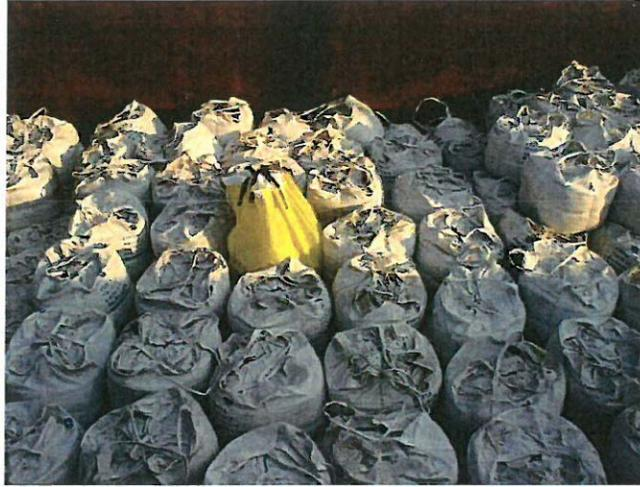
**Image 4 - "Super Sacks" in barge. The materials are highly dense, and so material piles do not exceed the side walls of the barges' holds, because the barges cannot carry that much weight. This picture likely shows a barge at full capacity for these dense alloys.**
