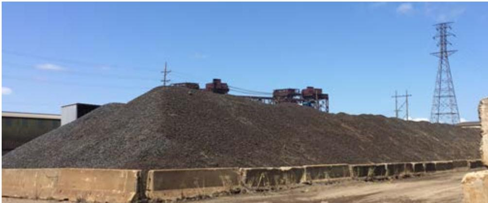
**Image 14 - Aggregate Pile - Pebble sizes range from 0.25 to 1.5 inches**
