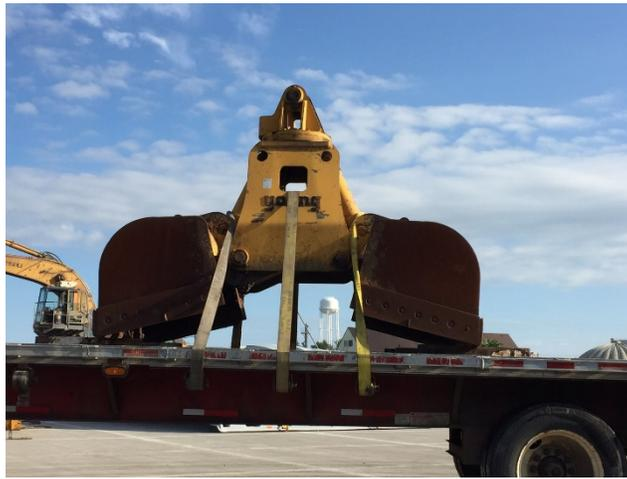
**Image 18 - Clamshell excavator attachment**
