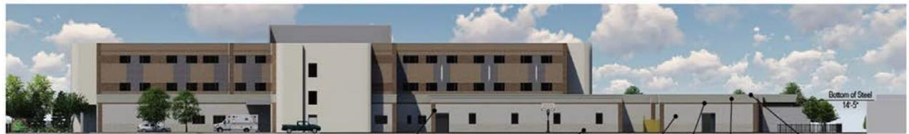
Running bond brick accent. North Elevation 12" High textured rock face stone. 8" High smooth-faced rock face stone. Soldier course brick. 4" High smooth-faced rock face stone. Cast stone parapet cap.
