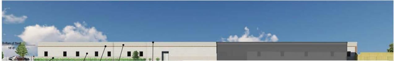
12" High textured rock face stone. 8" High smooth-faced rock face stone. Soldier course brick. 4" High smooth-faced rock face stone. Cast stone parapet cap.
