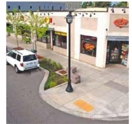
2 Corner and mid-block bumpouts, with landscape area that could be designed to reduce, slow down, and filter stormwater runoff.
