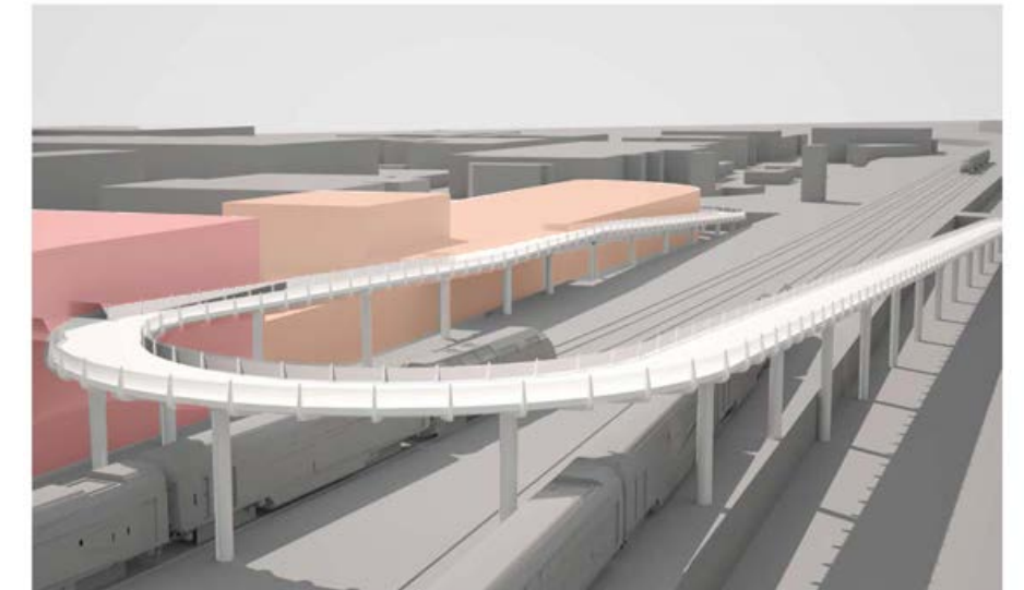
VIEW LOOKING SOUTH RAMP TO NORTH AT 5% SLOPE 23FT CLEARANCE
