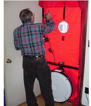
**ADDITIONAL INFO:** A blower door is a fan/door testing device that creates a controlled pressure difference between the inside and outside of a home by varying the speed of the fan. Leaky homes require higher fan speeds to produce a given pressure difference than do tighter homes. The blower door is useful in quantifying the degree of leakiness of a home (i.e., how “tight” the home is) and helps in identifying where leakage occurs, thereby directing additional air sealing work if needed.
