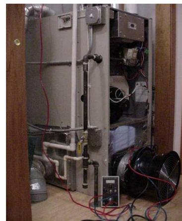
**Duct leakage testing** is performed using a Duct Blaster™ or equivalent type fan (shown image above). The fan is connected to the duct system at the air handler cabinet. With all the registers and grills temporarily sealed, duct leakage is measured by either pressurizing or depressurizing the duct system and measuring the fan flow. Duct leakage can be no more than 10% of system airflow when pressurized to 25 Pascals with the fan.
