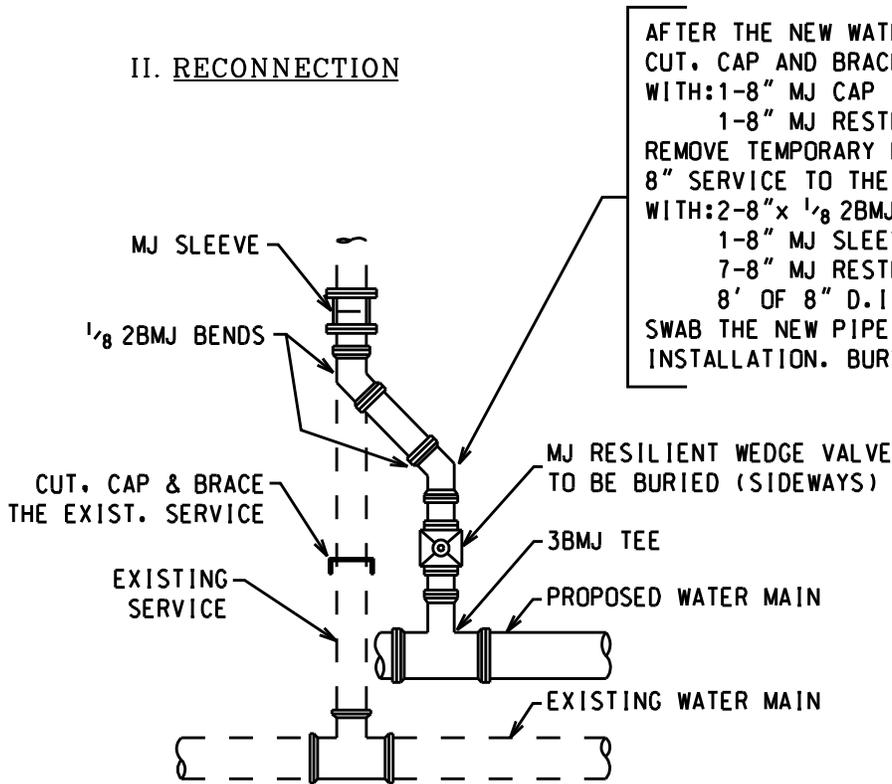
AFTER THE NEW WATER MAIN IS APPROVED, CUT, CAP AND BRACE THE EXISTING 8" SERVICE WITH: 1-8" MJ CAP
