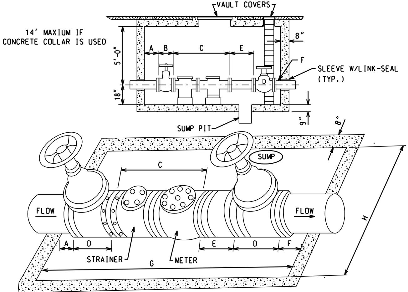
1" TAPS REQUIRED UPSTREAM AND DOWNSTREAM. ALL PIPES AND FITTINGS SHALL BE FLANGED AND SHALL CONFORM TO U.S.A. STANDARD A21.51-1965 (A.W.W.A.C. 151-65) AND SHALL HAVE ON OUTSIDE BITUMINOUS COATING OF EITHER COAL TAR OR ASPHALT BASE AND A CEMENT MORTAR LINING CONFORMING TO U.S.A. STANDARD A21.4-64 (A.W.W.A.C. 104-53).
