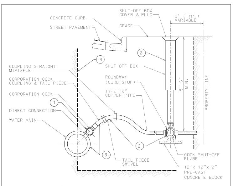
CONTACT CHIEF PLUMBING INSPECTOR (312-744-7017) TO COORDINATE WORK AND SCHEDULE AN INSPECTION. ALL WORK MUST BE INSPECTED/APPROVED PRIOR TO BACKFILL; FAILURE TO COMPLY WITH DWM REQUIREMENTS MAY INCREASE PROJECT COSTS TO VERIFY DWM STANDARDS HAVE BEEN MET.
