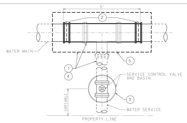
CONTACT DISTRICT SUPERINTENDENT TO COORDINATE WORK AND SCHEDULE AN ON-SITE MEETING PRIOR TO CONSTRUCTION. ALL WORK MUST HAVE FINAL INSPECTION/APPROVAL PRIOR TO BACKFILL; FAILURE TO COMPLY WITH DWM REQUIREMENTS MAY INCREASE PROJECT COSTS TO VERIFY DWM STANDARDS HAVE BEEN MET.
