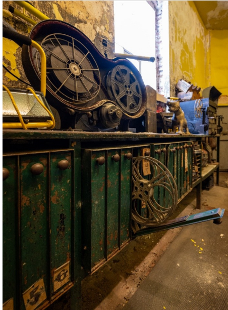
Though no longer in use, the projection booth retains vintage film reel cabinets and Peerless Magnarc projectors which produced light by an electric arc via combustion of carbon electrodes.
