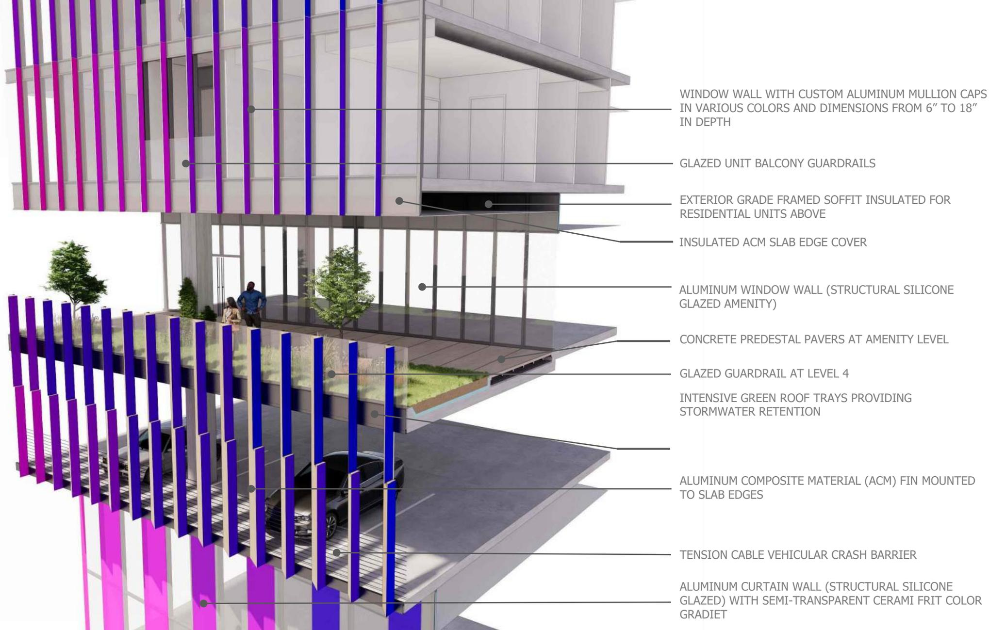
WINDOW WALL WITH CUSTOM ALUMINUM MULLION CAPS IN VARIOUS COLORS AND DIMENSIONS FROM 6" TO 18" IN DEPTH
