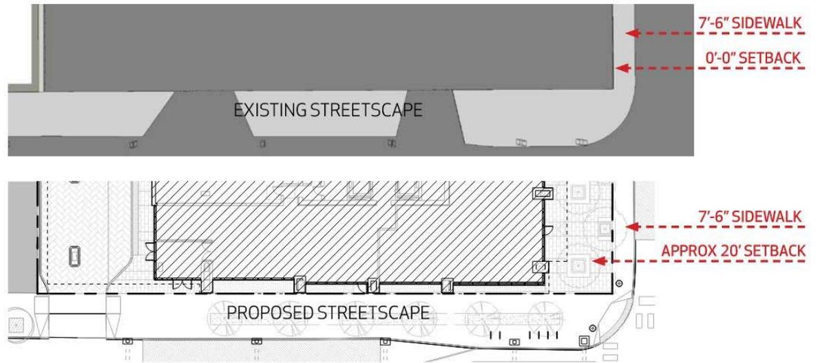
A strategic set back is proposed along Halsted Street to increase the size of the sidewalks due to adjacency with the high traffic corridor.
