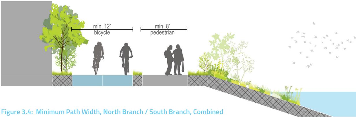
Figure 3.4: Minimum Path Width, North Branch / South Branch, Combined
