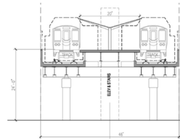
Figure 4.15: Center Platform Configuration
