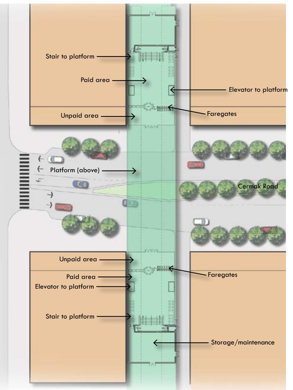
Figure 4.19: Cermak Road Green Line Station Side Platform Concept
