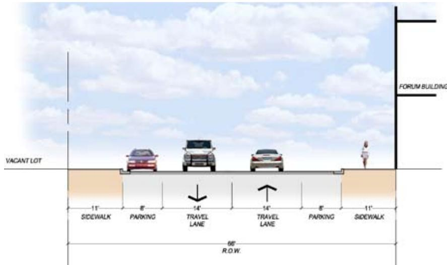
Figure 5.3: Existing Typical Section of 43rd Street between Prairie Avenue and Calumet Avenue
