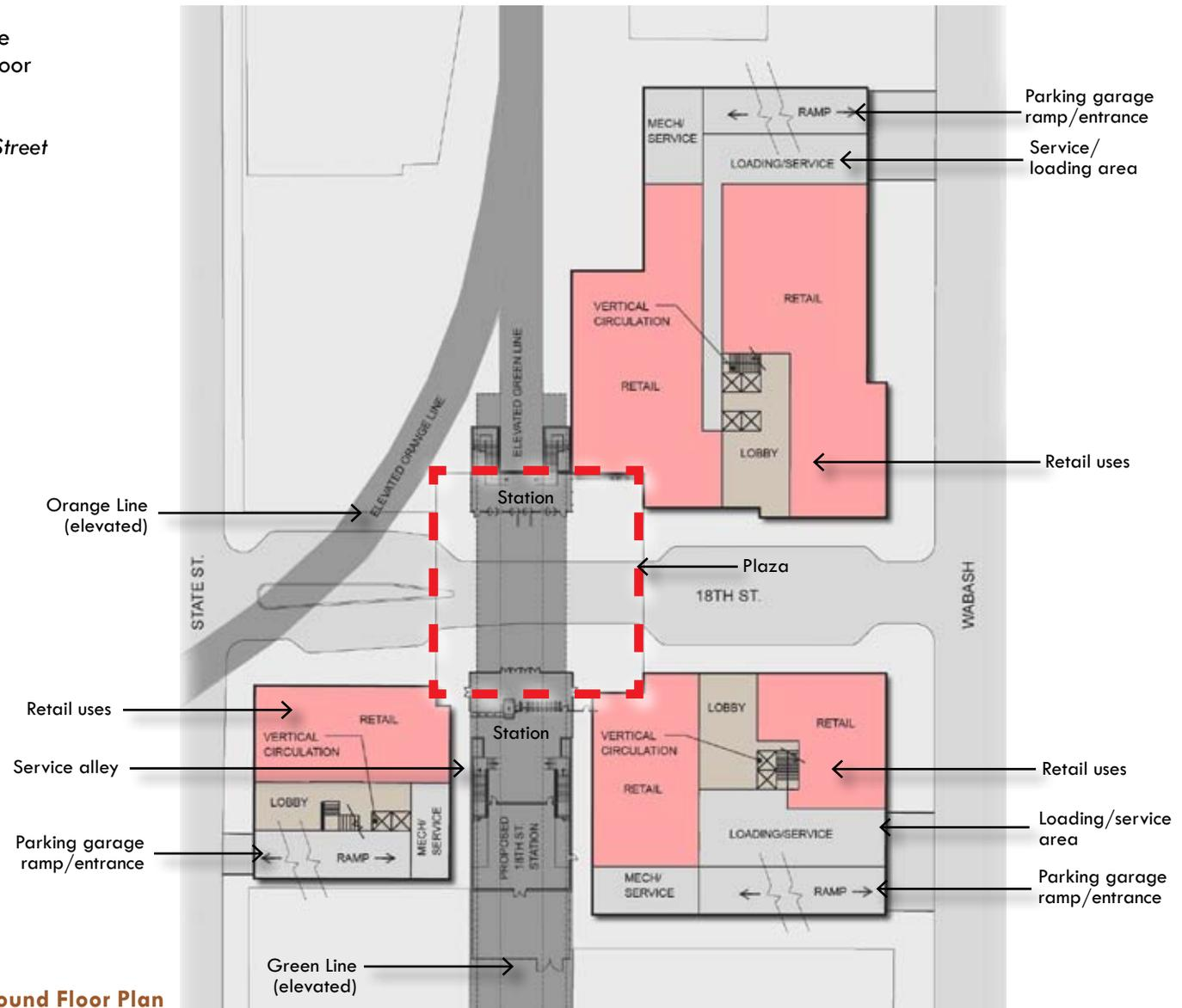
Figure 3.3: Ground Floor Plan
