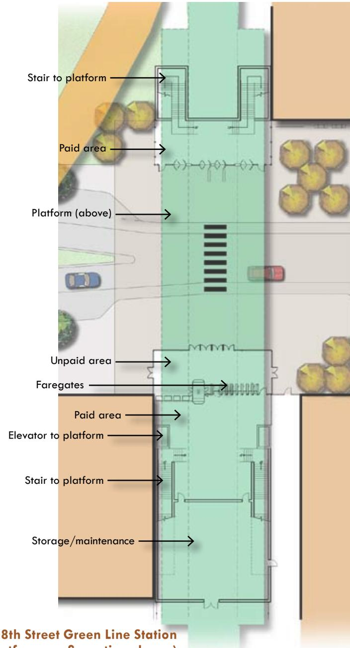
**Figure 3.10: 18th Street Green Line Station (side platform configuration shown)**
