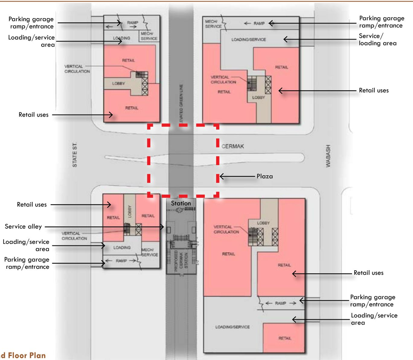
Figure 4.6: Ground Floor Plan
