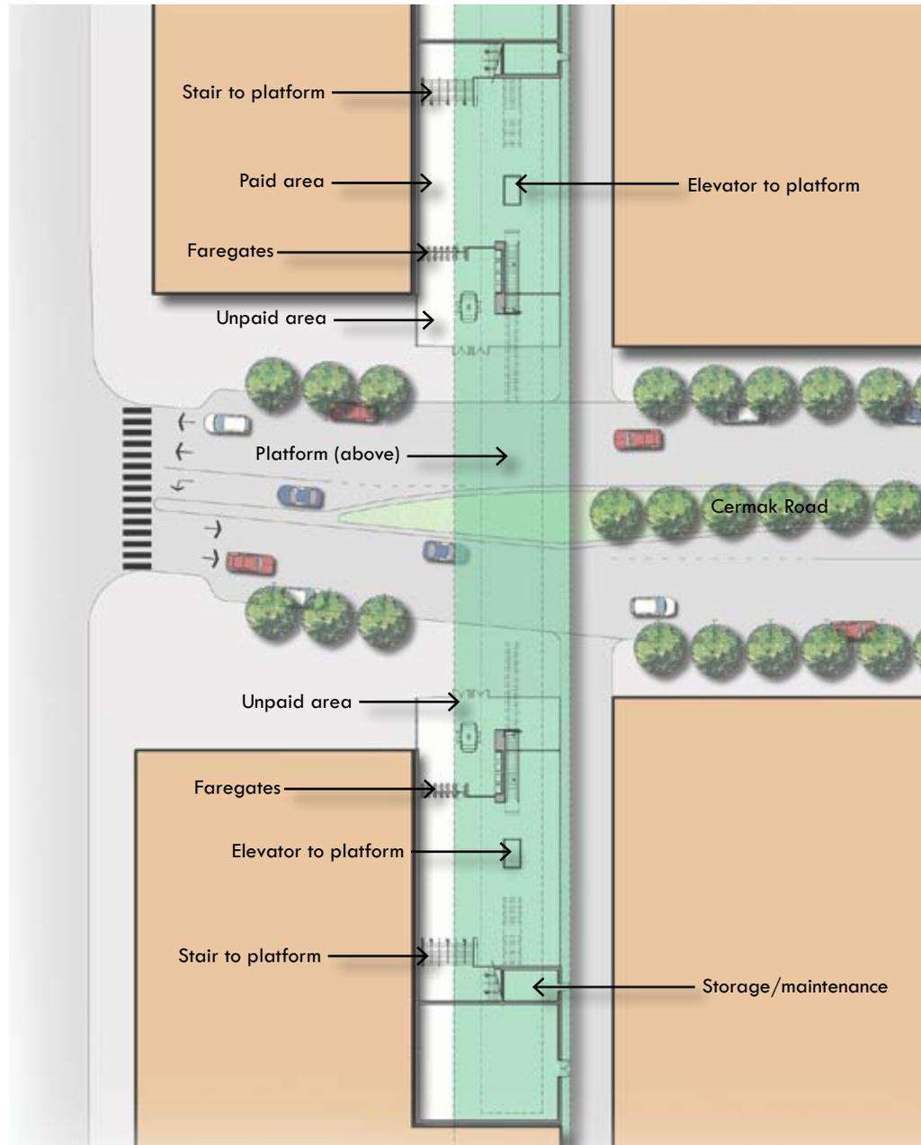
Figure 4.18: Cermak Road Green Line Station Center Platform Concept
