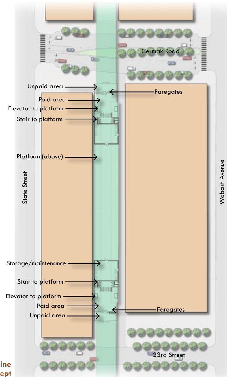
**Figure 4.17: Cermak Road Green Line Station Cermak to 23rd Platform Concept**
