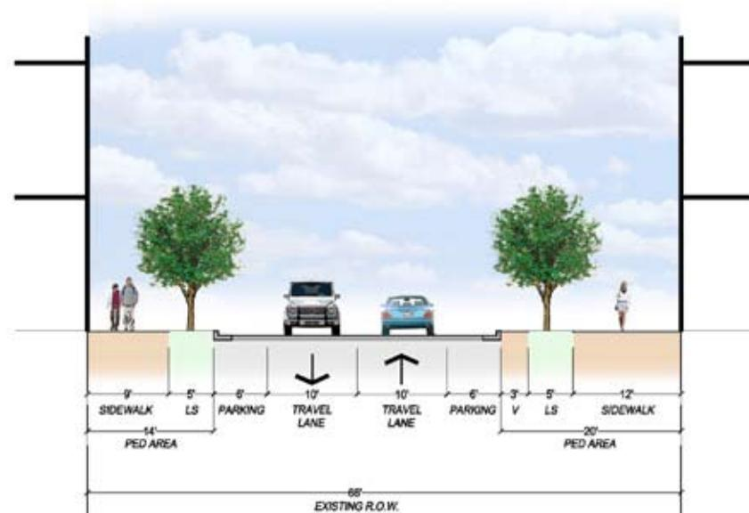
Figure 2.4: Existing Typical Section of Berwyn Avenue, East of the Red Line
