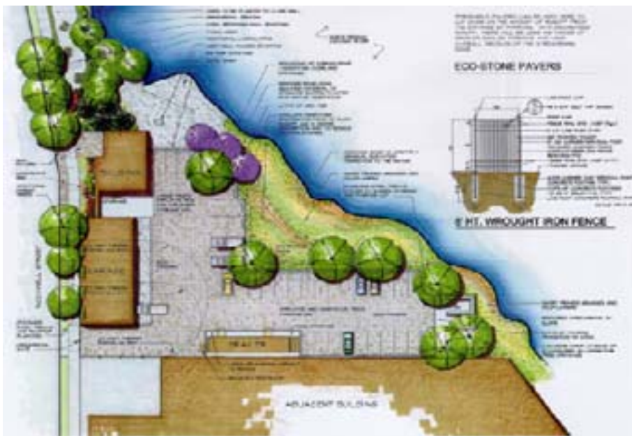
Figure 6.7 Example of riverfront industrial site utilizing riverbank recontouring, infiltration area, and porous pavers for stormwater management.
