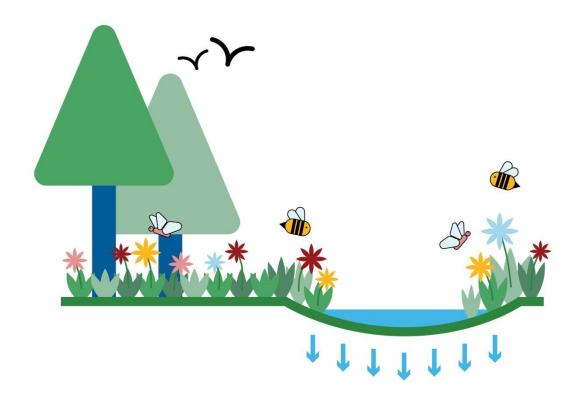
Green infrastructure (GI) collects stormwater from paved and unpaved surfaces to filter and absorb stormwater where it falls, reducing the amount of stormwater going into the sewer system.
