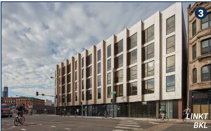
Undulating facade was designed to reduce glare from oncoming traffic for a better resident experience LINKT BKL
