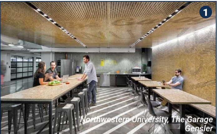
Flat floors and floor-to-floor heights allowed this parking garage to be repurposed as an incubator space.
