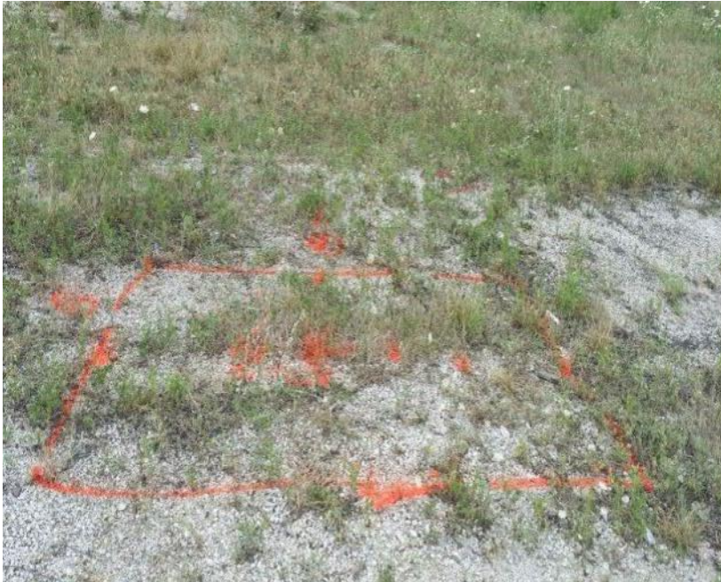
Photo 9: Closer view of the 6'X8" anomaly - potential UST.
