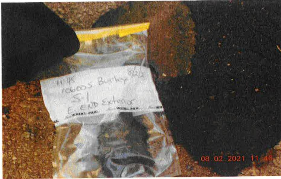
COMMENTS: Photo C- 11600 S. Burley, Sample #1, rubber roofing, NO Detect for ACM
