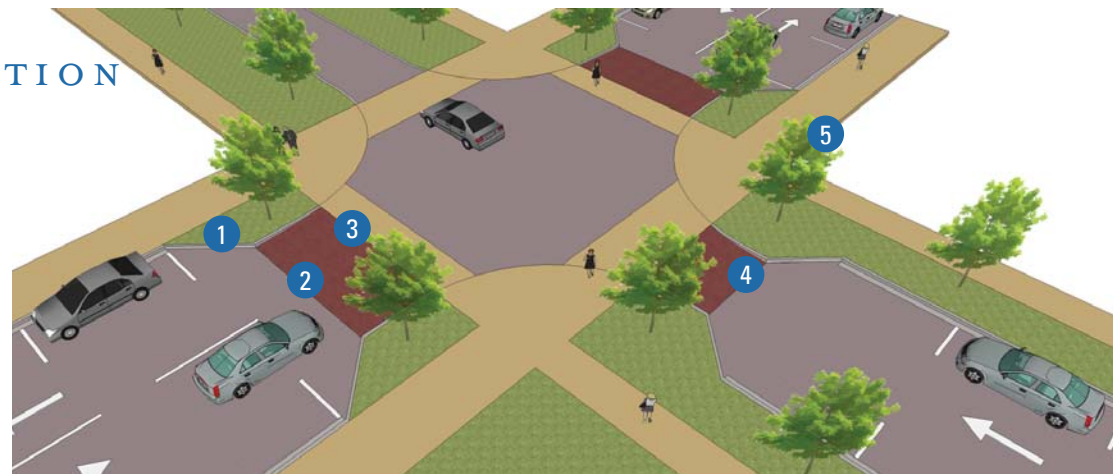
TYPICAL INTERSECTION OF 63 STREET (2 WAY STREET, ON-STREET PARKING) AND ONE WAY RESIDENTIAL STREET.
